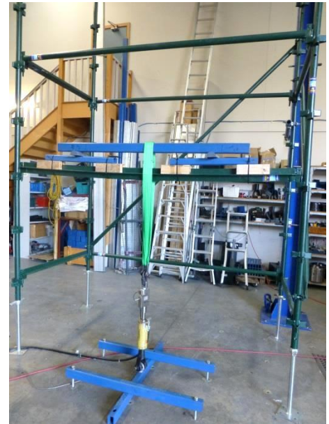
FIG.4 2.4M TRANSOM TEST SETUP
