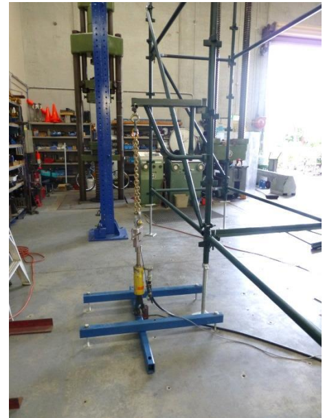
FIG.2 3 BOARD HOP-UP TEST SETUP
