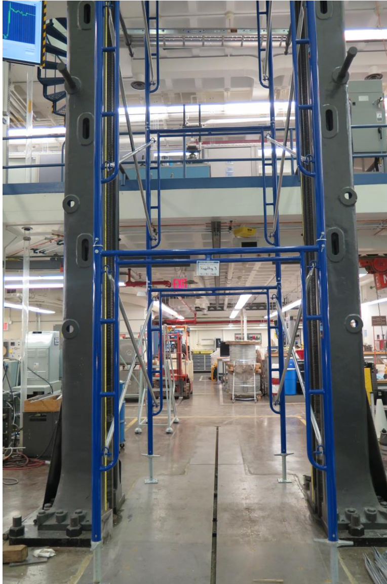
Before test (#3: 5' X 19' scaffold assembly)
