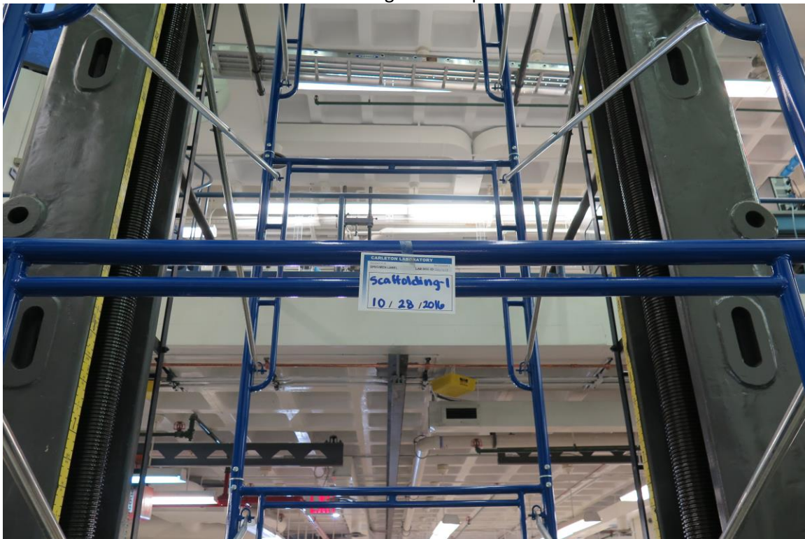
Before test (#1: 5' X 19' scaffold assembly)
