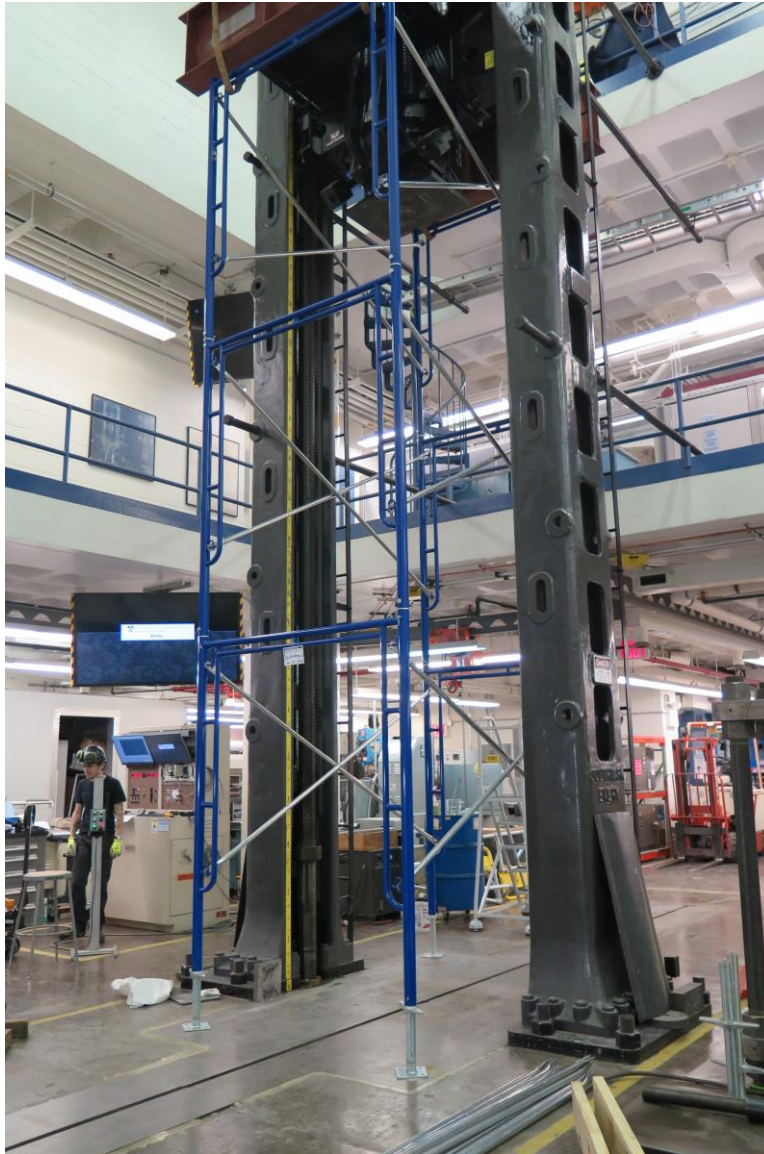
Before test (#2: 5' X 19' scaffold assembly)
